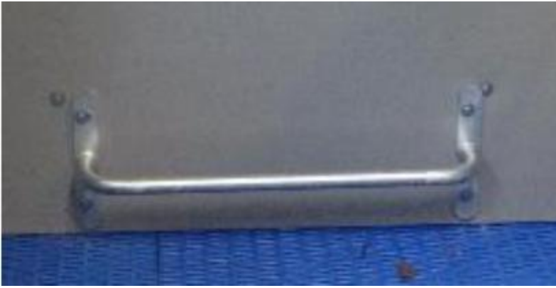
Figure 13 : Barre anti-écrasement ; © RANNOU G, Elevage B, 2018
