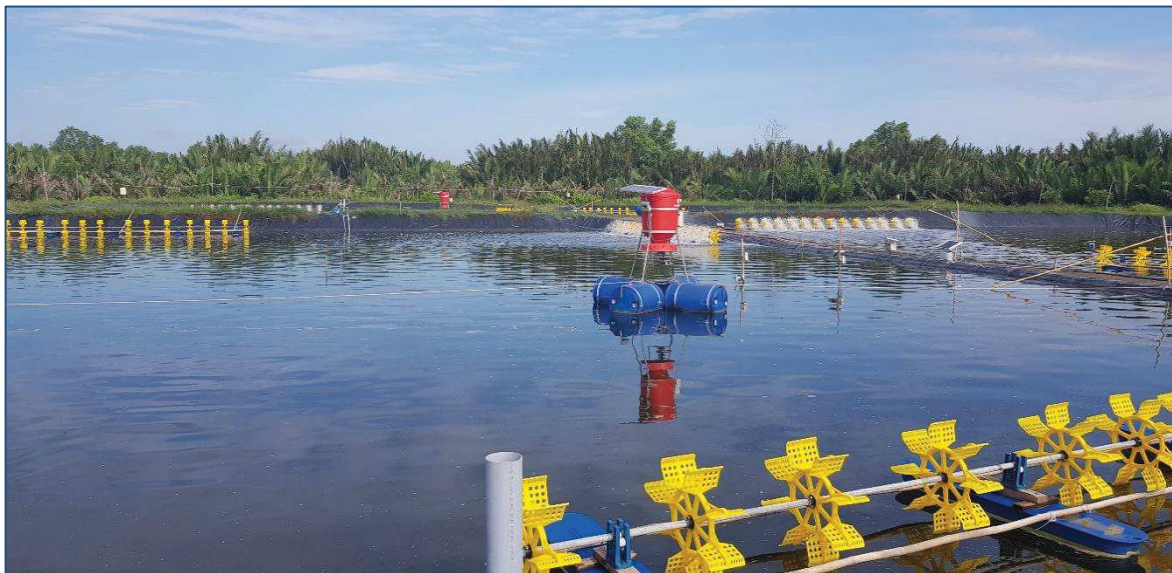
Appendix VIII: Picture of a grow-out pond at daytime. An automatic feeder can be seen in the center, and one paddlewheel per pond is working in the background (Jean-Benoît Darodes de Tailly, 2019, Nhà Bè, Vietnam).
