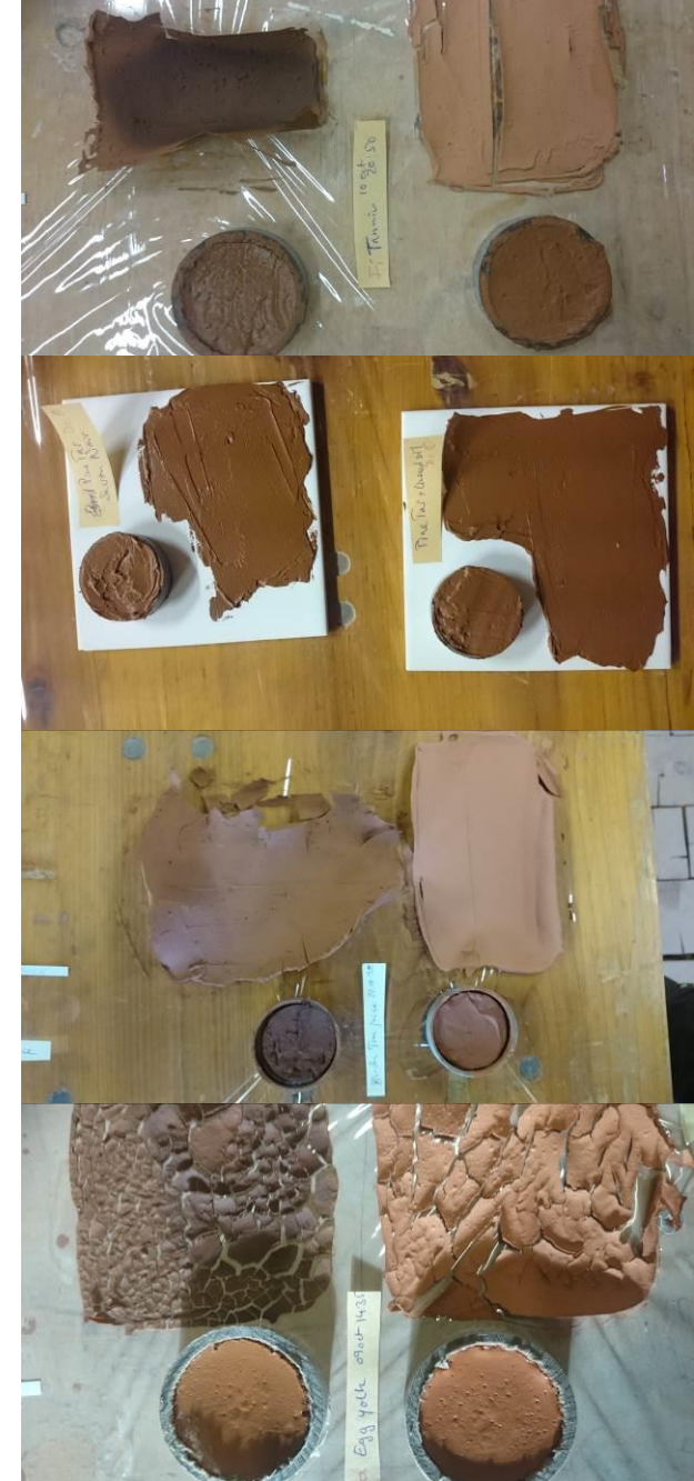
Above: samples from top to bottom show mixes with Tannins, Pine Tar, Birch Tree Juice and Egg Yolk
