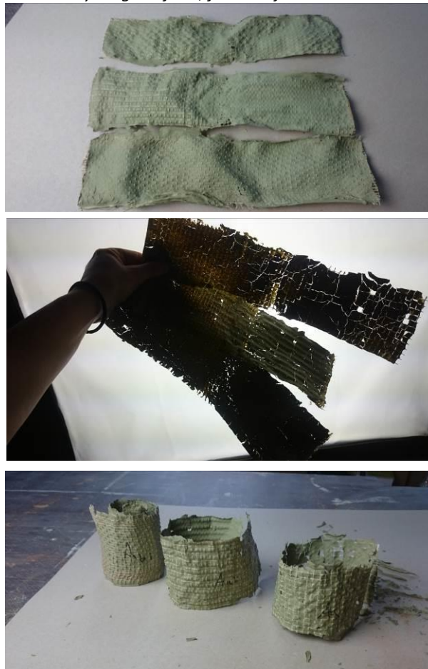
Top to bottom: Green clay on glass fibre, flax and jute mesh
