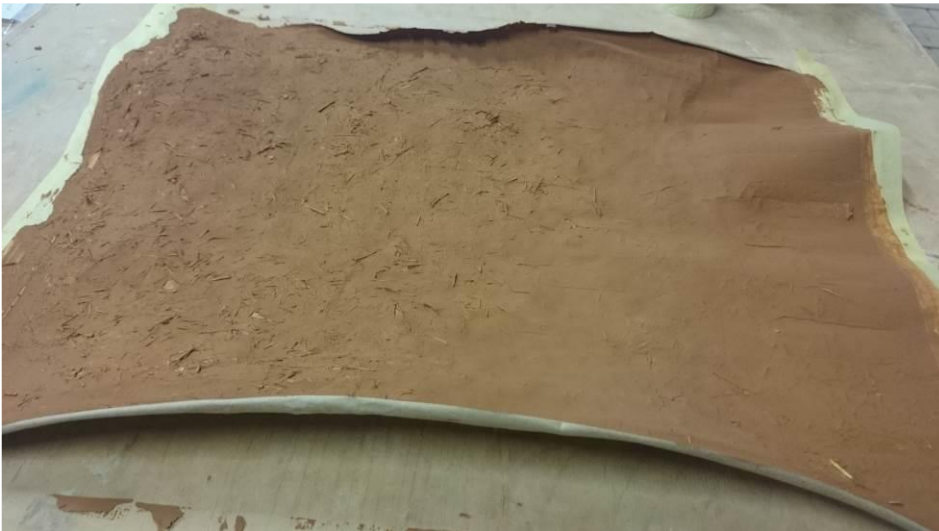
Below: Clay paste applied to recycled paper and left to dry
