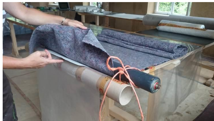
Top left: 8kg steel roll tied down with twine, used to roll dry paper
