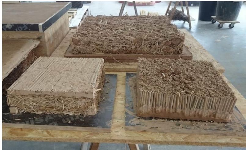
Making thermal and acoustic insulating wall coverings while .....
