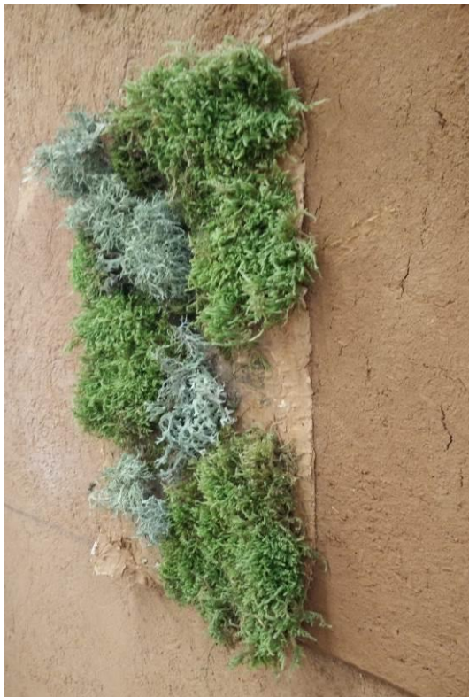
A clay wallpaper piece was painted with Kefir, and moss and lichen left for a few days sitting on the sample to grow into it. The sample was hung on the wall sprayed for a few days with water, then forgotten about and removed in the course of a general refurbishment two years later, with the moss doing fine whereas the lichen had fallen off.
