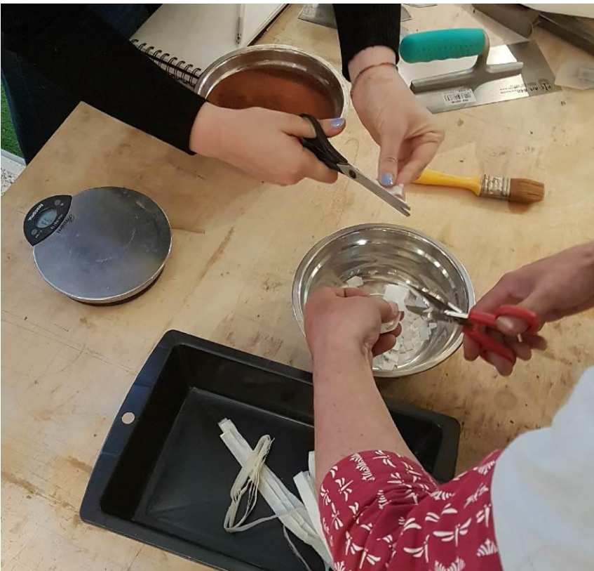
Cutting Washi-paper into small pieces before soaking in water and using the blender on it
