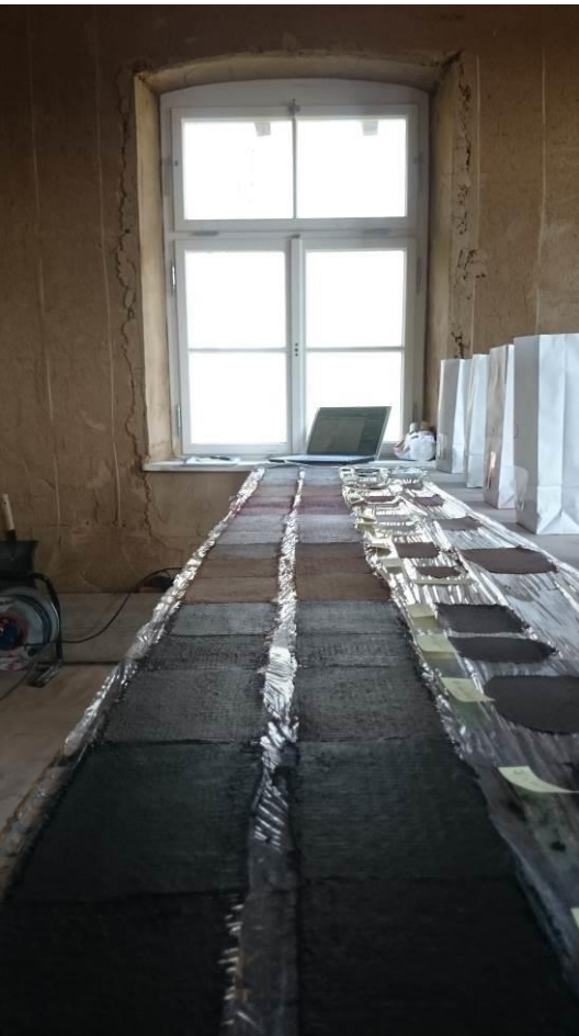
Worktop set up for testing clays fibres and additives
