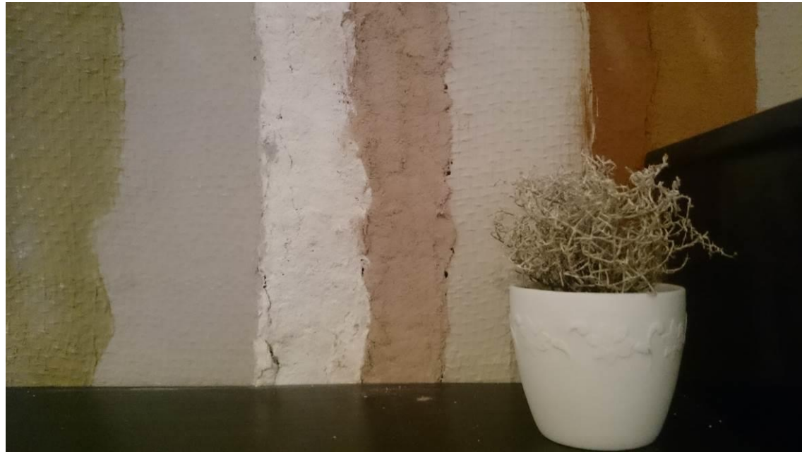
Sample with various Estonian clays (Test 9)
