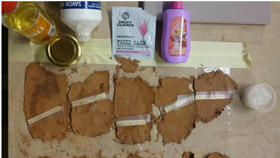
Test 7 A variety of chemical laxatives and smoothing agents for hair was tested
