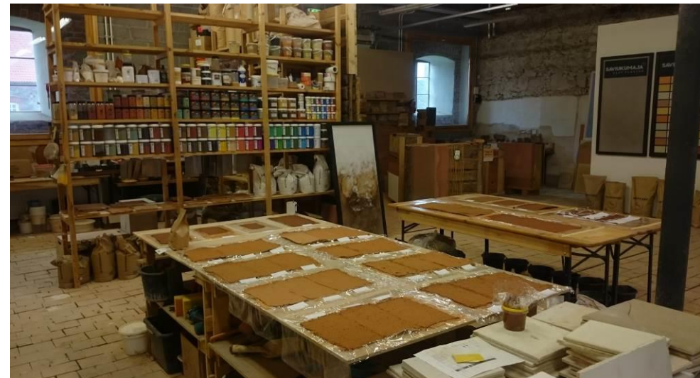
Samples testing fibrous mixes with and without fibre mesh as a reinforcing substrate
