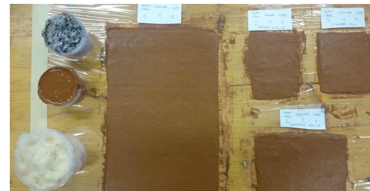
Below: various fibres mixed into samples to achieve a better grading of fibre for clay to attach to
