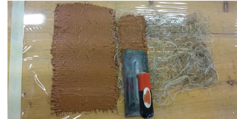
Below: various fibres mixed into samples to achieve a better grading of fibre for clay to attach to
