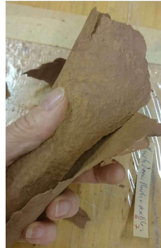
Test 10 result using synthetic fibre in clay mix
