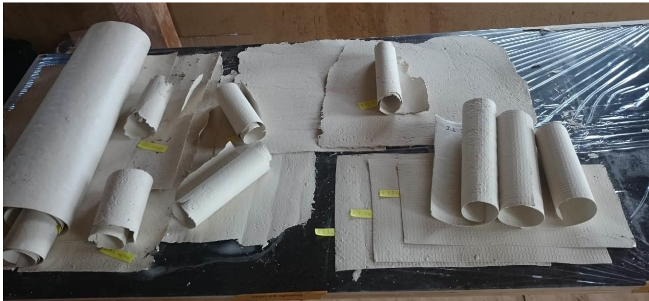
Collection of samples deemed ready to be used on walls, based on Capsil® clay, various fibre and mineral components
