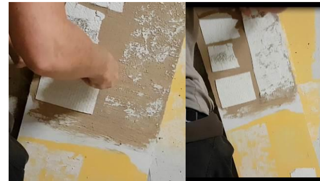
Top: Lifting a ca. 0.5m 2 of a 12.5mm gypsum fibre plasterboard (ca. 10kg) by pulling on the jute mesh wall paper sample of 0.01 m 2 area of connection.
