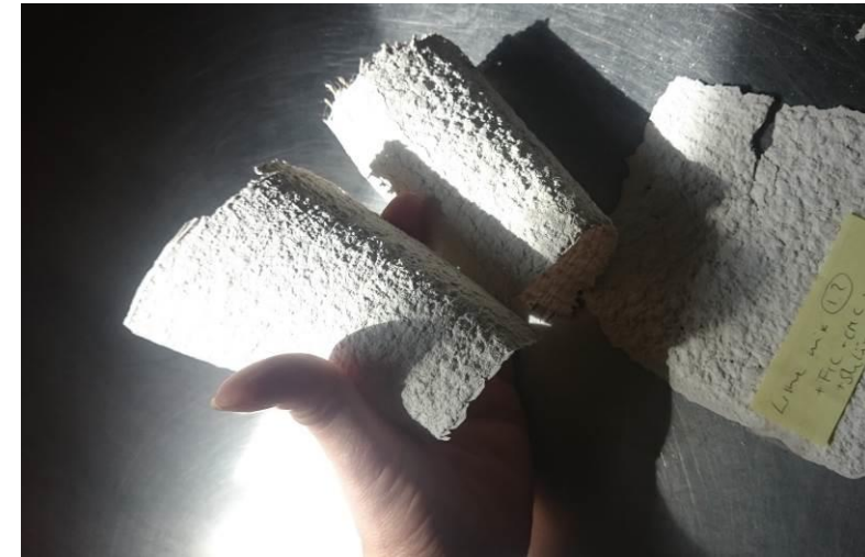
Ssamples with variations of lime and other mineral additives
