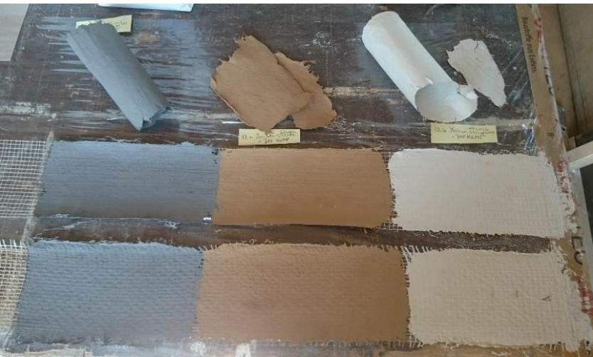
Samples of Lasko, Baulehm and Capsil® with and without mesh
