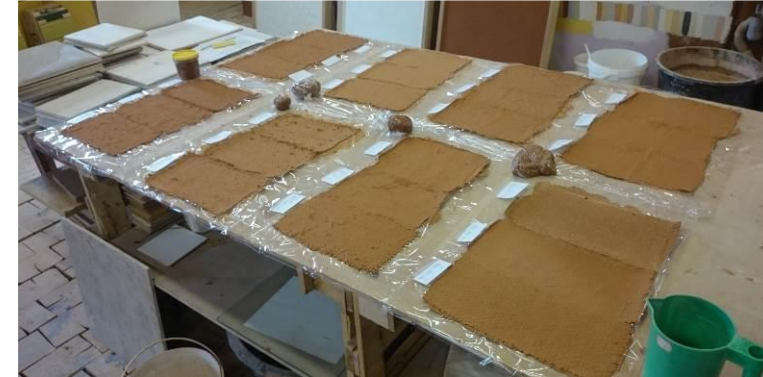
Same clay mix applied to mesh and loose fibre
