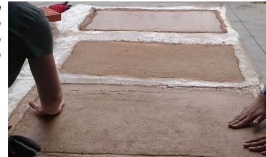
Samples in the making Top: 1 mesh Middle: 2 mesh Bottom: 3 mesh
