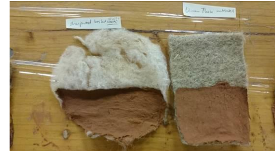
Test 8 results from boiling fibre in acid and lye
