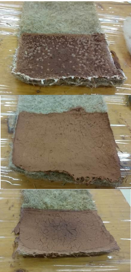
Top to bottom: Linen felt boiled in alkali, in water, in acid
