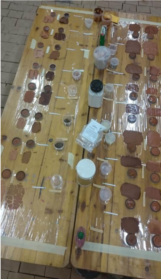
Set up for various agents tested on red Latvian and light red Latvian earth
