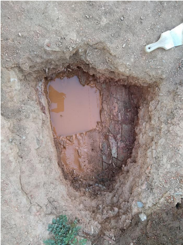
← Digging the ground in Mourão to find the depth at which the rocky ground is found. This depth determines the depth of the foundation and is likely to differ from area to area, even within the same village. (Picture taken in August 2018)
