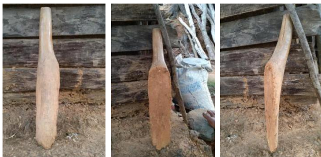
'Pattnem' used by the owner-builders in Salgini village to build their rammed-earth houses.
