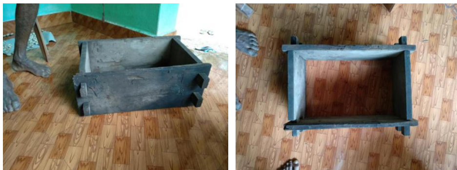
Image 77 and Image 78: Mason Babuso's adobe-brick mould.
