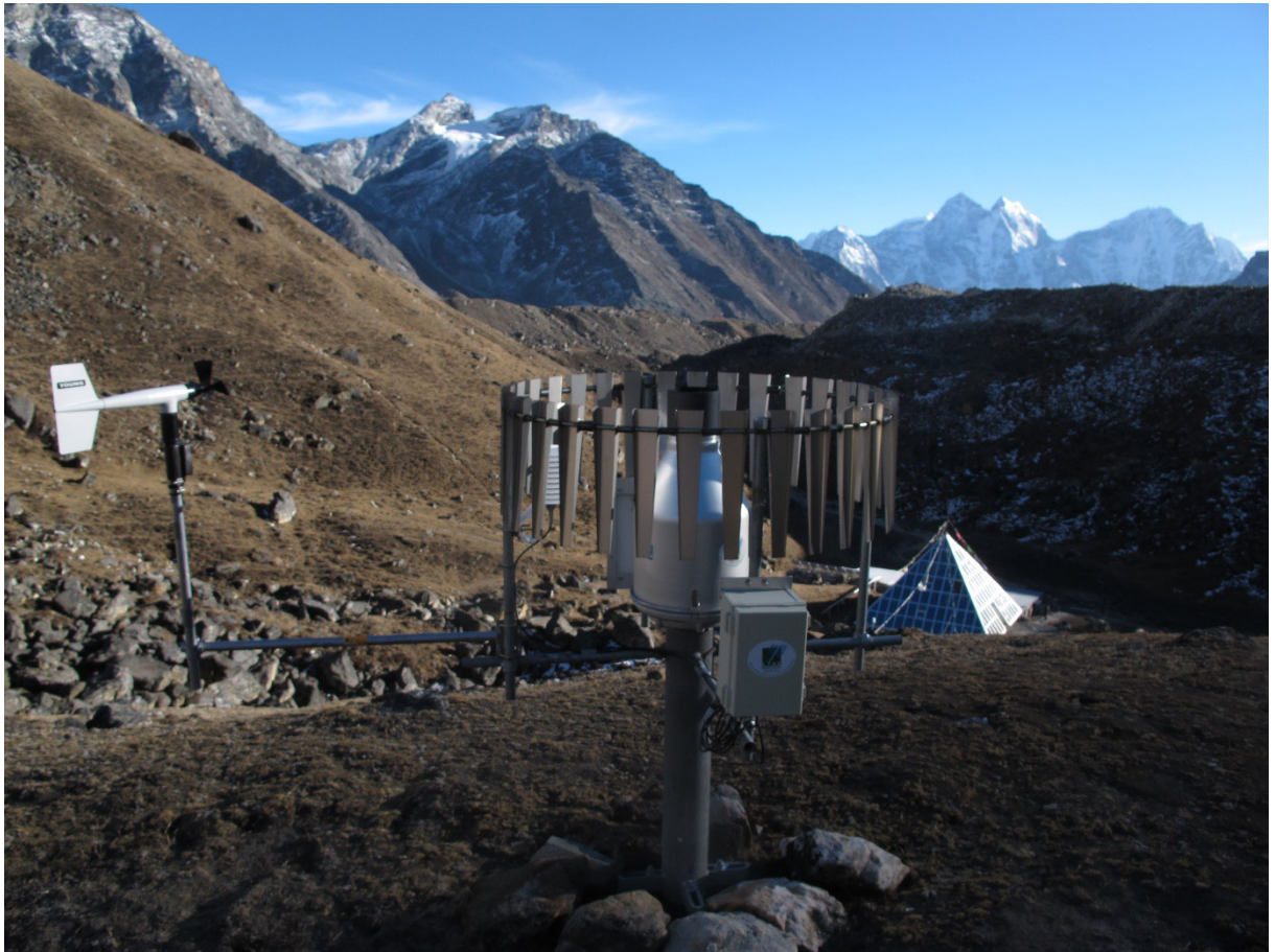
Figure 4: Photo of the Geonor T-200B (22/11/2015, ©Wagnon) recording precipitation at 4993 m a.s.l. and used in this dataset
