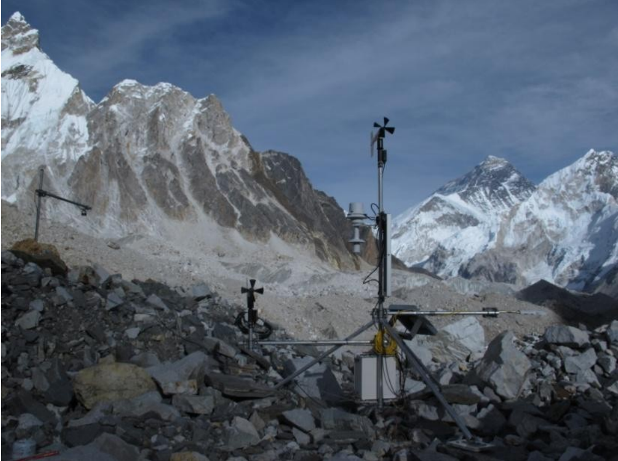
Figure 3: Photo of the AWS CN-5360 (27/11/2015, P. Wagnon)
