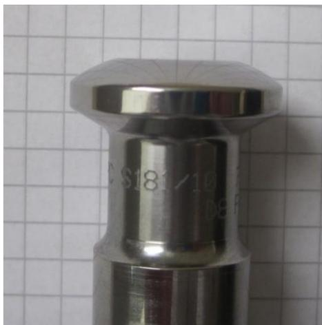
FIGURE 28: TETE D'UN POINÇON
