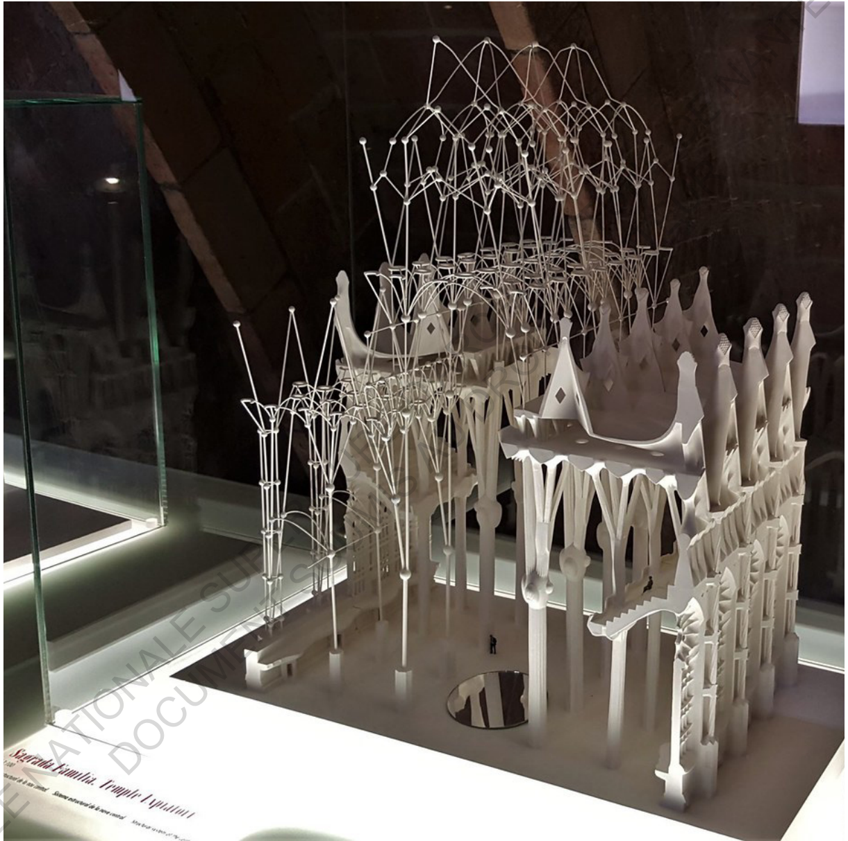
Upside-down model of the Sagrada Familia created by Gaudí Source : flickr.com
