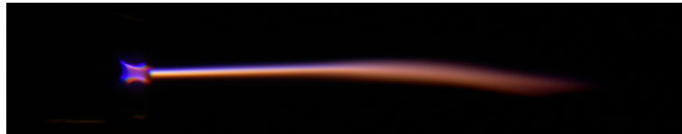
(a) Argon plasma jet with 0.7% of N_2 , 9.4 cm long.
