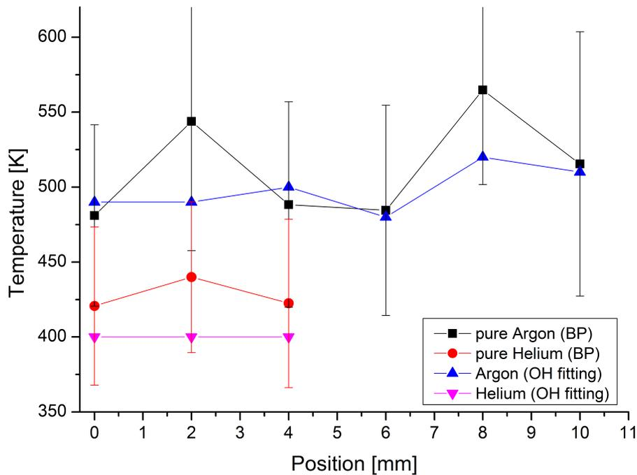
Figure 5.5: Pure Argon and Helium plasma jet OH rotational temperature for different position from the needle electrode. *BP* and *OH* fitting mean that the temperature is estimate by the Boltzmann plot and the fitting respectively.
