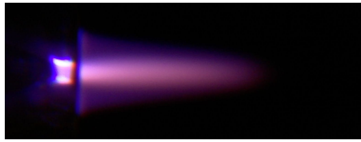
(a) Helium plasma jet with 0.7% of O 2 , 3.0 cm long.
