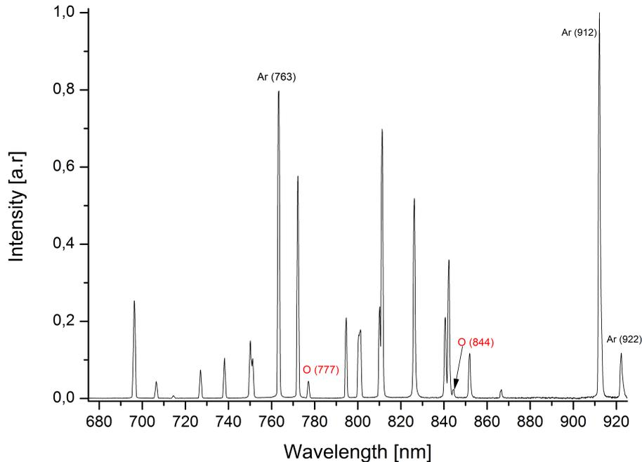
Figure 3.3: Spectrum of the Argon APPJ from 650 to 930 nm.
