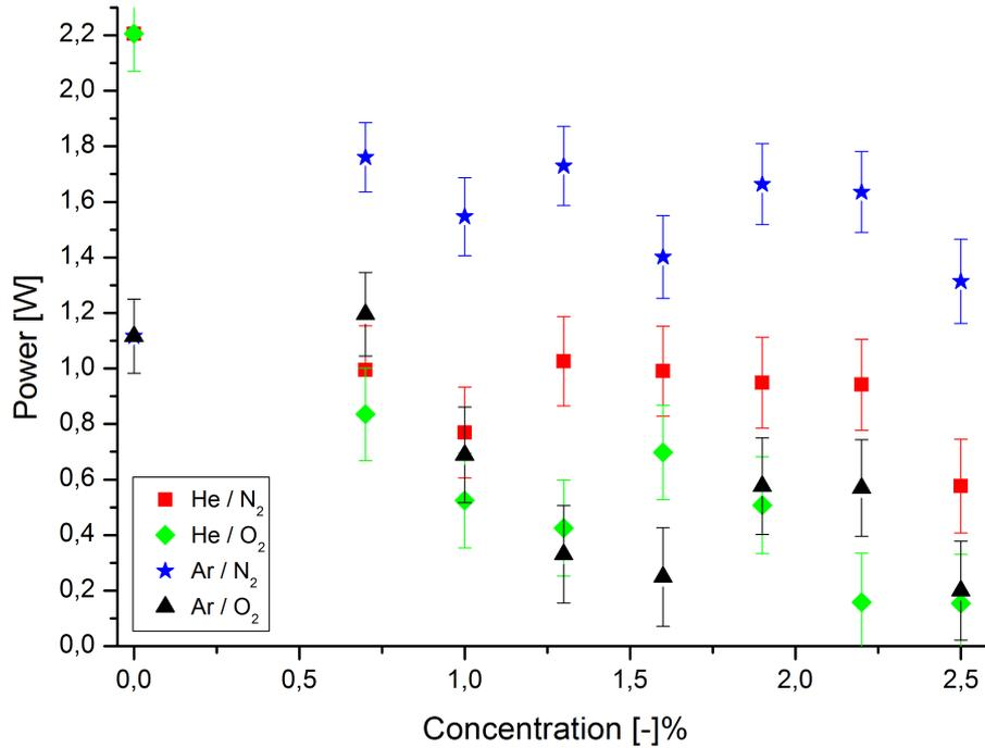
Figure 4.4: Plasma dissipated power for different gas mixtures. For all this measurements  $I_{RMS}=0.9$  A.
