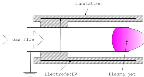
Figure 1.4: Schematic of the plasma jet device developed by Cheng *et al.*[3].
