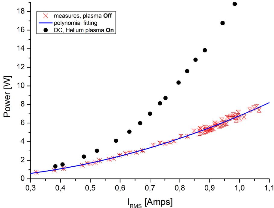
Figure 4.2: Plasma dissipated power calculation method. This example is from a Helium plasma jet without second electrode.
