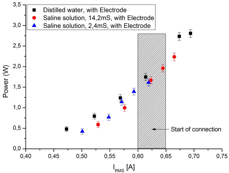
Figure 6.3: Dissipated power Helium plasma jet for different solution conductivities.
