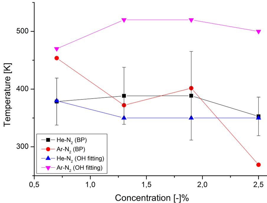
Figure 5.6: OH rotational temperature for different gas mixture concentrations with Argon and Helium. The errors for the Ar-N<sub>2</sub> gas temperature from the Boltzmann plot is not drawn because the values are too big to be realistic.
