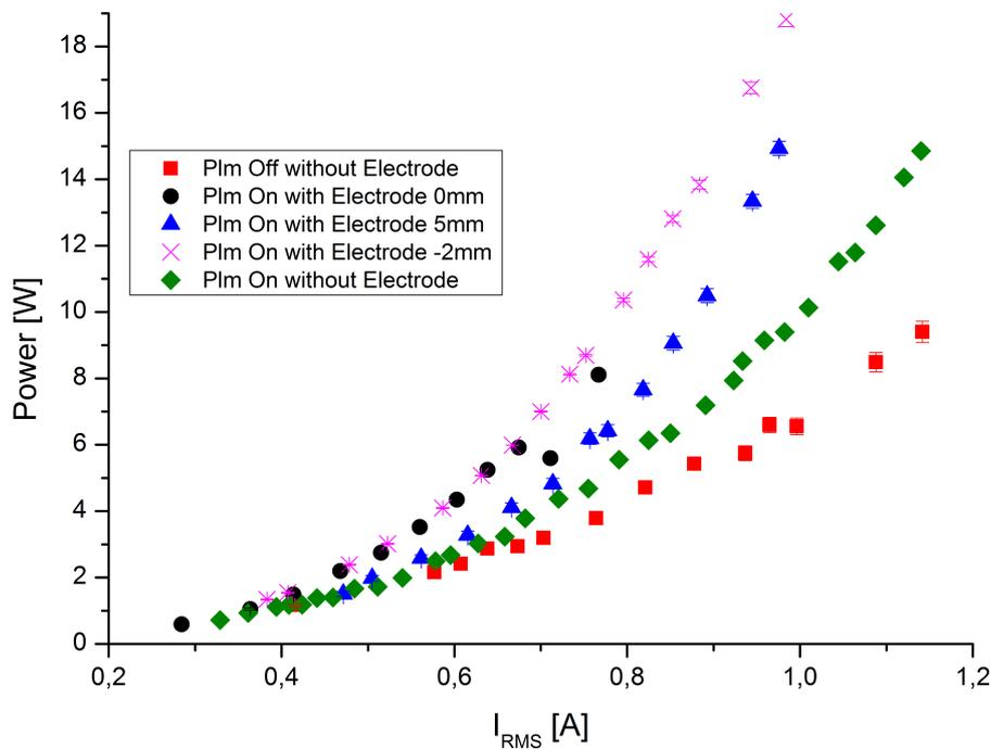
Figure 4.5: Influence of the electrode for the power measurement of a Helium APPJ.
