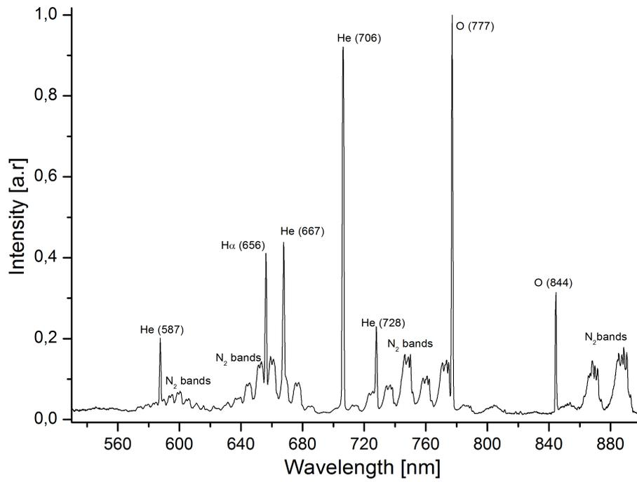
Figure 3.5: Spectrum of the Helium APPJ from 520 to 920 nm.
