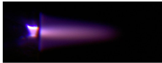
(a) Helium plasma jet with 0.7% of N_2 , 4.1 cm long.
