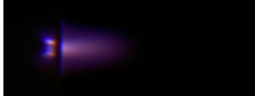
(b) Helium plasma jet with 1.3% of O 2 , 2.1 cm long.
