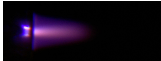
(b) Helium plasma jet with 1.3% of N_2 , 3.1 cm long.
