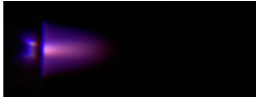
(c) Helium plasma jet with 2.5% of N_2 , 2.3 cm long.
