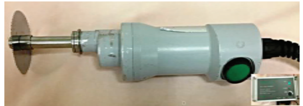
Fig. 1: The hand-held electrical saw with an oscillating blade used in this experimental study (with its electronic box).
