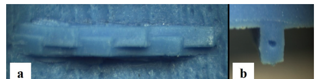
Fig. 2: Shape of profiles (casts of the false starts): (a) Saw 1: alternating of concavities and convexities; (b) Saw 2: concave profile.
