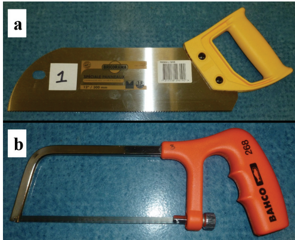
Fig. 1: Handsaws selected for this study: (a) universal saw; (b) rip saw.
