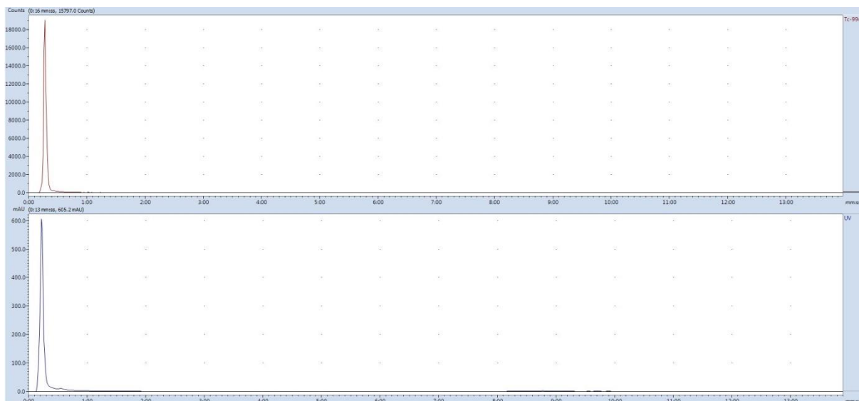
Figure 21 : Radiochromatogram HPLC of ^{99m}\text{Tc} -trensox (total counts in red and mAU in blue)
