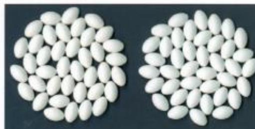
Left: SheffCoat™ TF, applied as a 15% dispersion in water to a 6% weight gain at a tablet bed temperature of 42-44°C
