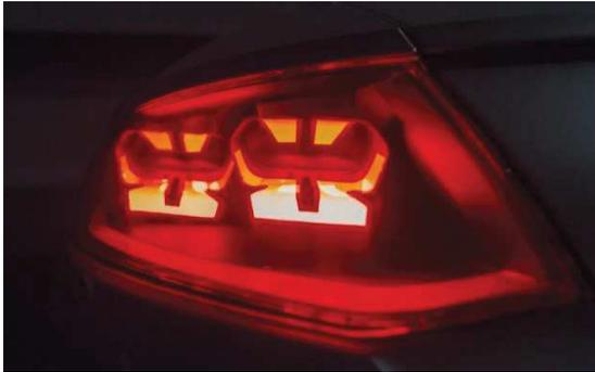
Three-dimensional LEDs will soon be entering series production. “In flexible OLEDs, the substrate material is simply a film – instead of rigid glass,” says Berlitz. “We can use this to design totally new shapes and achieve completely new, three-dimensional effects. This combination of aesthetics and highly innovative technologies is something we will continue to push in future, because OLEDs offer us even more progressive design options,” says the lighting engineer with visible glee.
