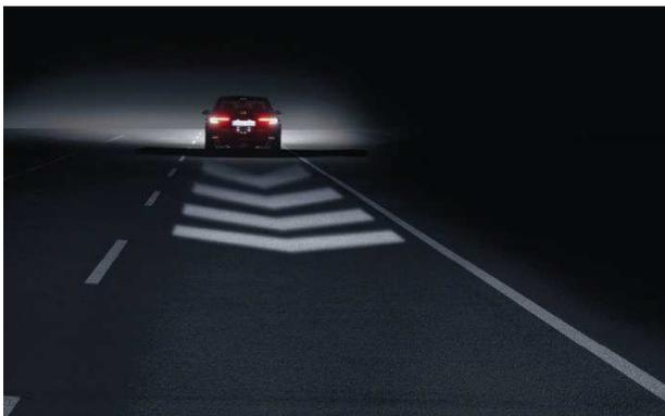
At the heart of the new front headlamps is a high-power laser which illuminates a matrix of almost half a million micromirrors. Their edges are only a few hundredths of a millimeter in length and each one can be individually tilted up to 5,000 times per second. “In future, we won’t
