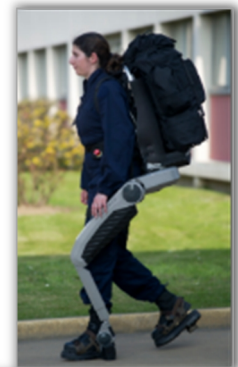
Figure 3 : Héraclès® de RB3D (Source INRS [18])
