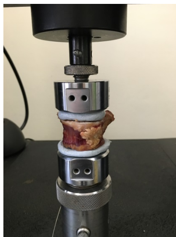
Fig 1 : Loading apparatus for mechanical testing of the vertebral specimen in compression.
