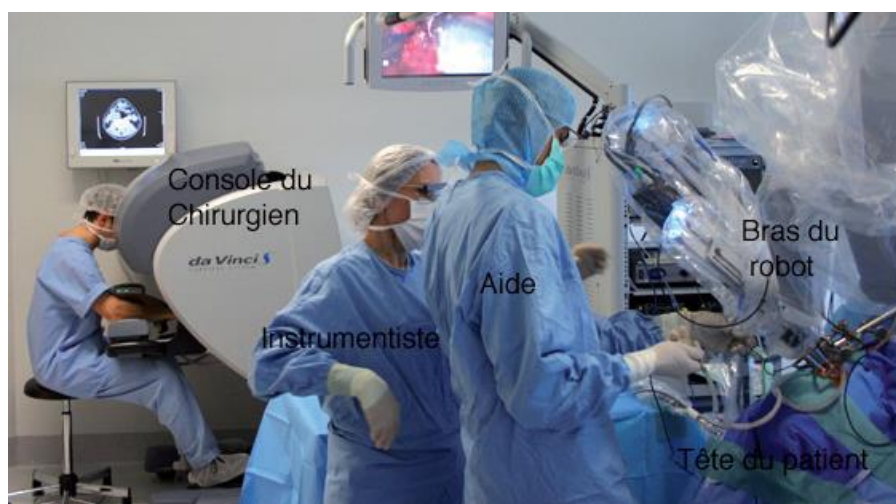
Figure 24: Installation du Robot Da Vinci®
