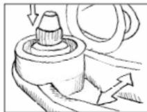
4 Snap eyepiece closed. (The bottle stays in Dispenser until empty. Repeat installation only on receipt of a new bottle)
