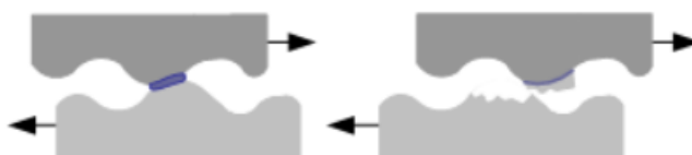
Figure 2.13: Adhesion wear mechanism as result of rubbing of two surfaces [35].
