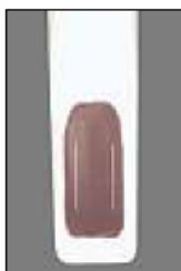
Light from green LEDs illuminates the membrane (Figure 4). A camera measures the reflected light (Figure 5) and the corresponding CRP concentration is displayed on the Analyzer screen.
