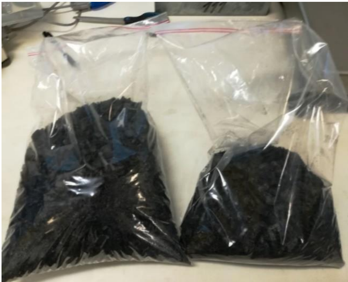
Figure 23: Biochar applied inside the bioreactors
