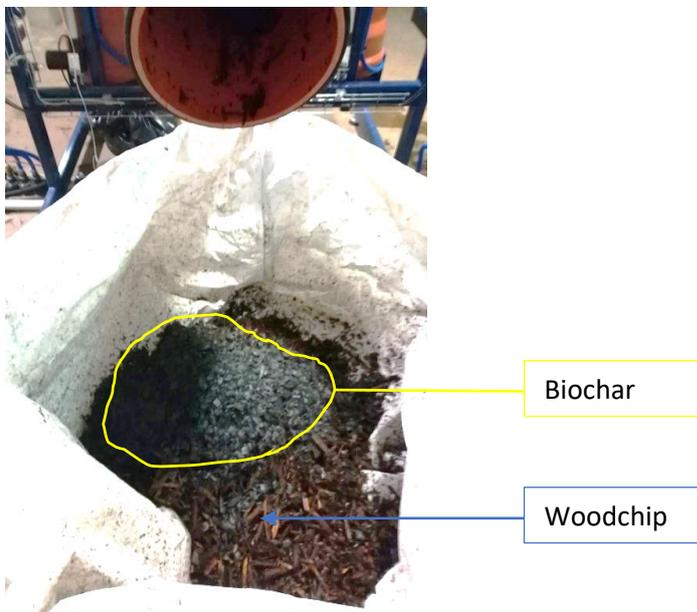
Figure 27: Emptying a bioreactor and addition of biochar
