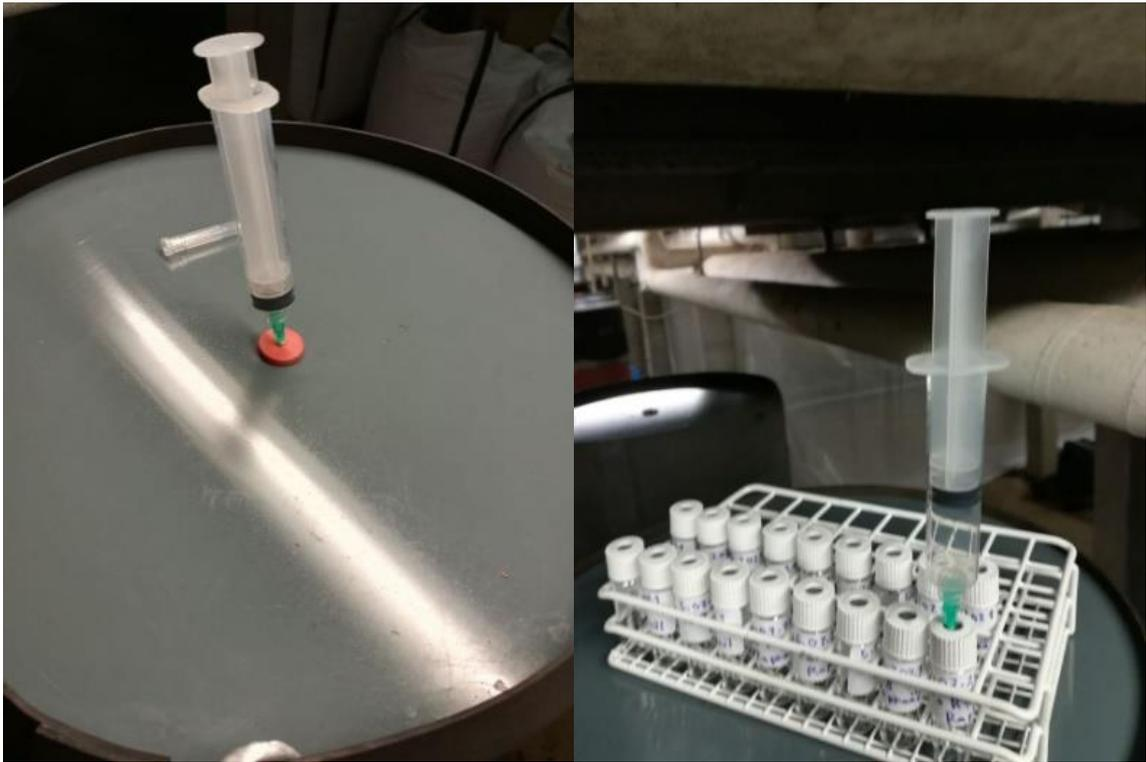
*Figure 21: Nitrous oxide sampling*
