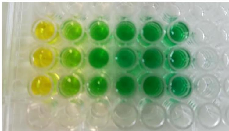
Figure 18: Prepared ammonium samples for the spectrophotometer
