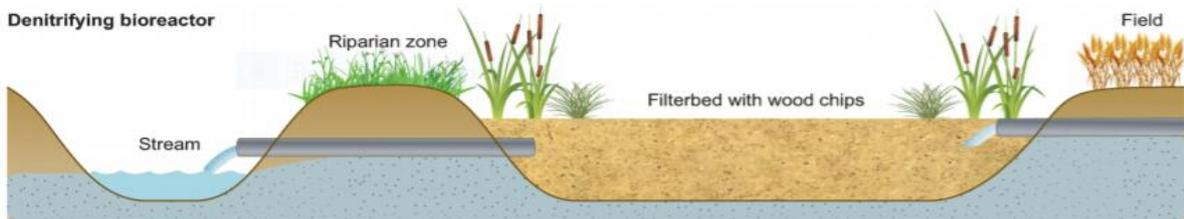
Figure 4: Woodchip bioreactors from Hoffmann et al.,2020
