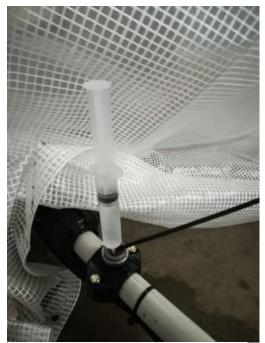
Figure 16: Water sampling at the INLET
