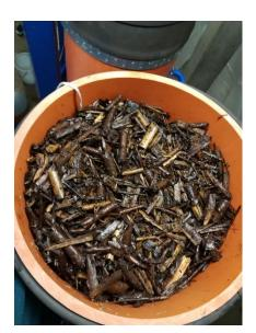
Figure 13: Willow woodchips within a bioreactor
