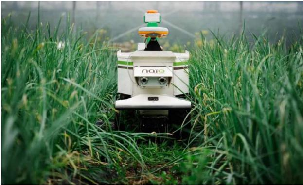
Figure 17 : Robot OZ 440 - Guidage GPS-RTK (GOFAR, 2020) [19]
