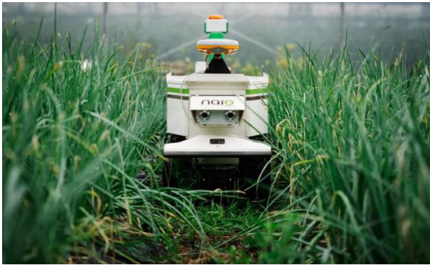
Figure 17 : Robot OZ 440 - Guidage GPS-RTK (GOFAR, 2020) [19]
