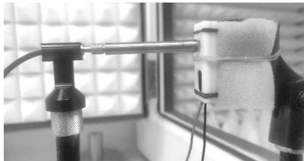
Figure 120 - BR system N ° 2 – Setup for measuring the SPL at port output
