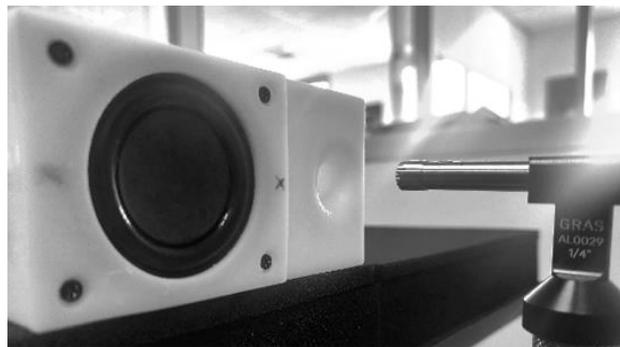
Figure 64 - BR system N° 1 – Setup for qualification of turbulences created by ports designs
