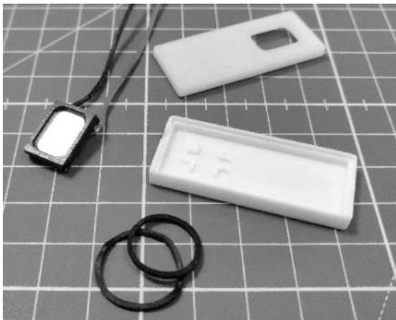
Figure 17 – Sealed enclosure N ° 2 - Assembly elements
