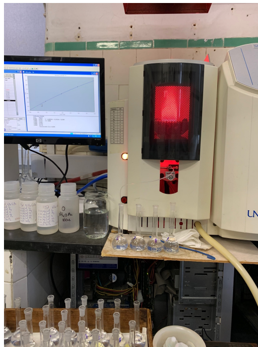
Figure 2.4: Reading of the Cations concentrations with the atomic absorption spectrophotometer of ISA
