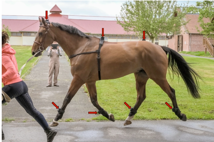
Figure 1. Horse equipped with EQUISYM® system, composed by sensors placed on the head, the withers, the pelvis and the 4 cannon bones (indicated by red arrows).
