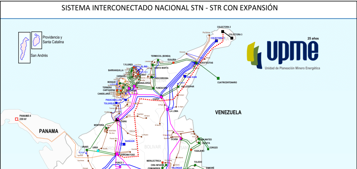
Figure 3.3. Prospective expansion map of Colombia's National Transmission System (STN) and Regional Transmission Systems (STRs) with a 2033 horizon. Source: UPME (2019a). Note: The projected transmission lines in La Guajira include the 500kV high voltage lines between the Colectora 1 substation –to be constructed– and Cuestecitas –located in the vicinity of El Cerrejón mine– as well as the HVDC line projected to carry the energy generated in Alta Guajira to the Cerro Matoso substation, from where it could be transported to Panama.
