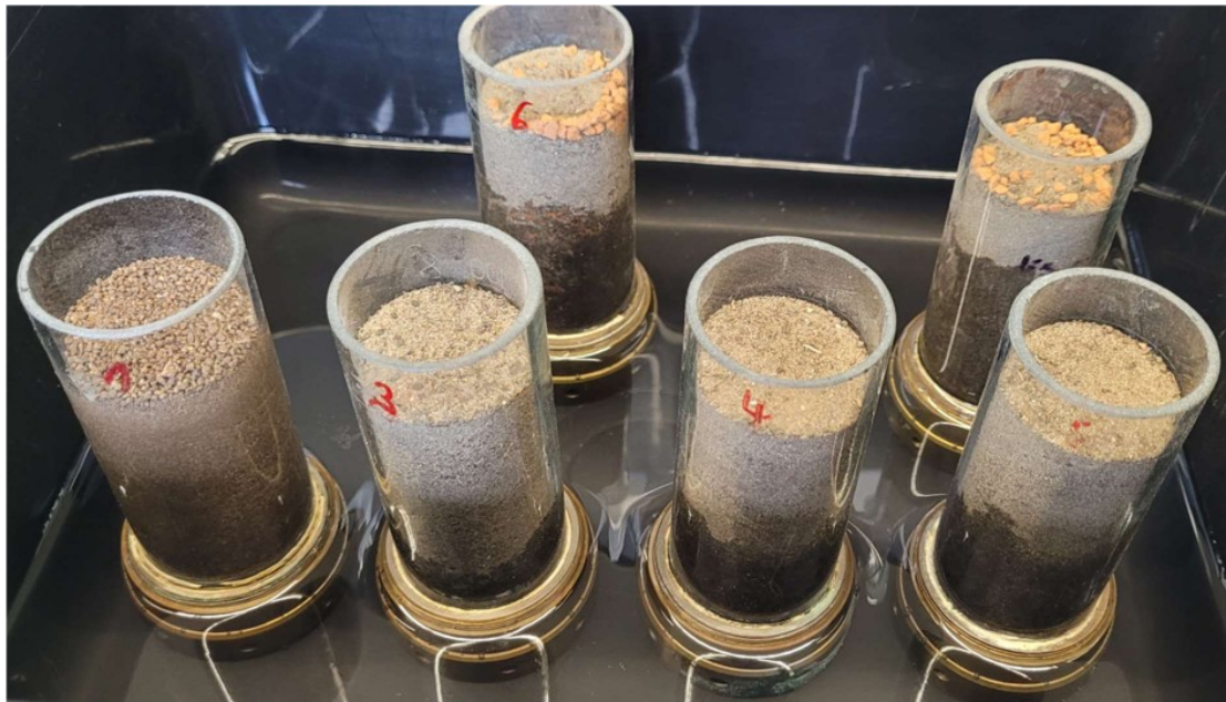
Figure 8: Measurement of the water holding capacity of the soils without and with 8% of iron sludge addition (front and back row, respectively) according to ISO 14238:2012 Appendix A: air dried soils were packed at a density of 1.2 to 1.3 Mg m -3 in glass cylinders with perforated base plates, transferred to a water bath until the soil columns were water saturated and, after drainage of the free soil water, weighted fresh and after drying at 105°C (26-04-2023).
