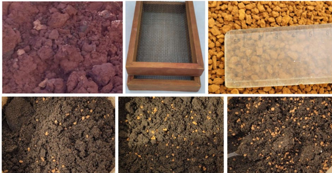
Figure 3 : Iron sludge before and after drying, crushing and sieving to particle sizes between 2 and 4 mm (upper row) and sewage field soil with iron sludge addition of 2, 4 and 8 % dry mass (lower row from left to right).
