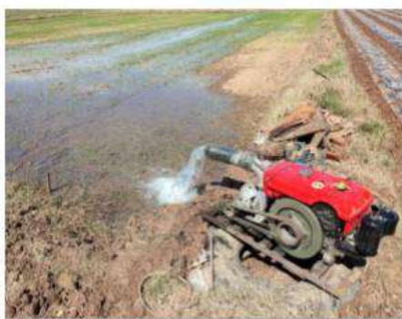
The water is coming directly from a borehole (Toul between Put and Nou). It is an irrigation operation of a rice plot, but the same system can be found for other crops in this area. The difference for rice plot is that water supply goes directly from the pump to the field, whereas pipes are generally used for vegetables.
