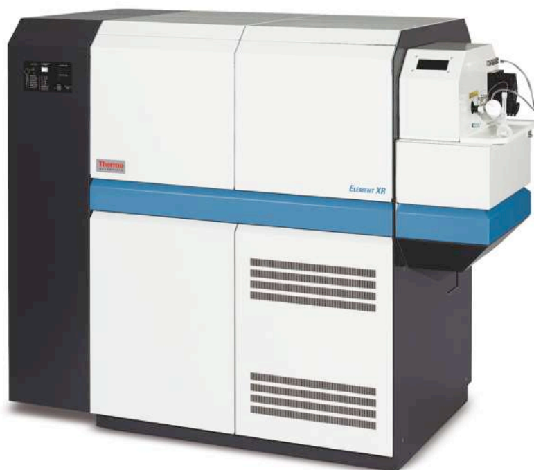
Illustration No. 22: ICP-MS instrument ELEMENT XR used for sample analysis. Source: https://chemistry.olemiss.edu/icp-sfms/
