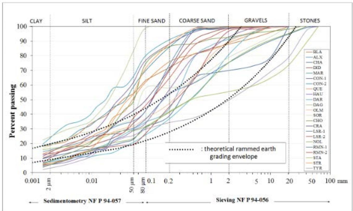
**Figure 5: A comparison between the theoretical grading envelope from Houben et al. [33], and grading curves of 23 samples from French vernacular rammed earth buildings measured in the present research program**
