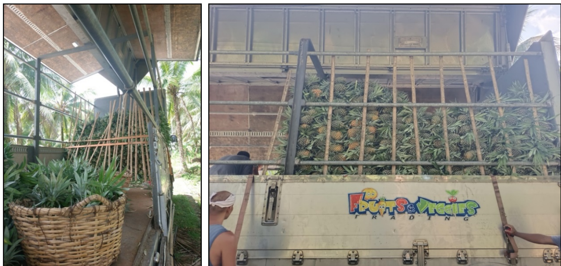
Figure 64. Slatted bamboo used as protective barriers within the transport vehicle, Camarines Norte, Philippines, 2023.
