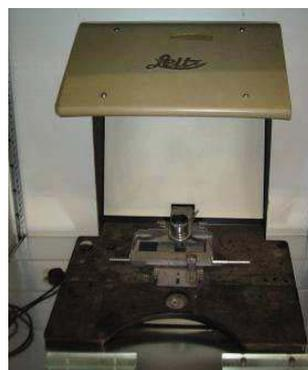
Figure 48: Trichinoscope
