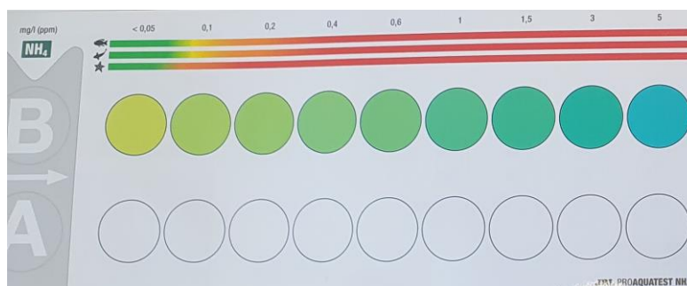
Figure 19: Colour chart for comparison of samples tested, here for the element NH 4 . B = blank sample. A = sample with reagent. Comparison of the two colours of the samples following the colour chart and where the colour between the blank one and the tested one appears identical, the corresponding concentration is recorded (Source: JBL GmbH & Co. KG, n.d.)
