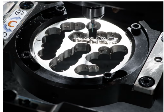
Figure 2: Disque de Titane grade 5 ø 98,5mm Dental Machine®
