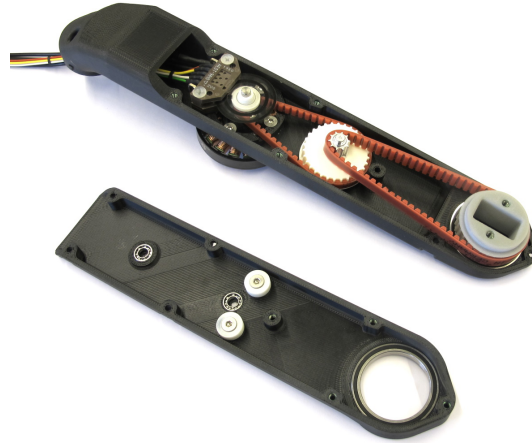
Fig. 24: Opened lower leg actuator of Bolt.
