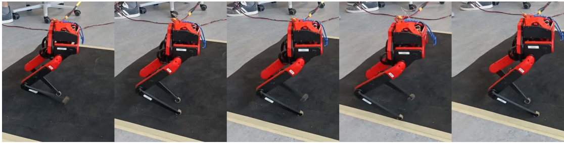
Fig. 18: Real Bolt walking with CaT at a speed of 0.0 m/s. Each image is separated by a time step of 1.0 s.
