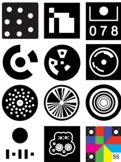
Fig. 1. Various types of coded targets used in industry
