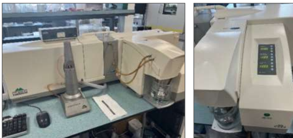
Figure 3.5 Malvern Mastersizer2000 Laser diffractometer (left) using a Hydro2000MU dispersion unit and water as dispersant. (right)
