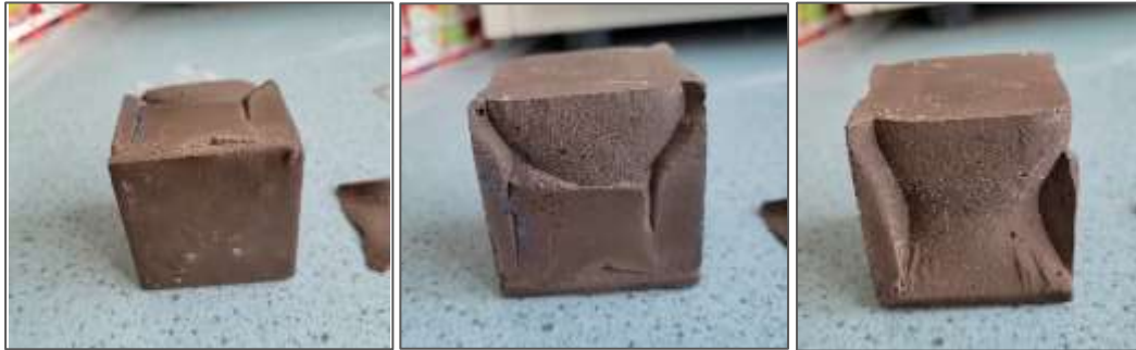
Figure 4.14 CC9F cubes broken in a vase shape.
