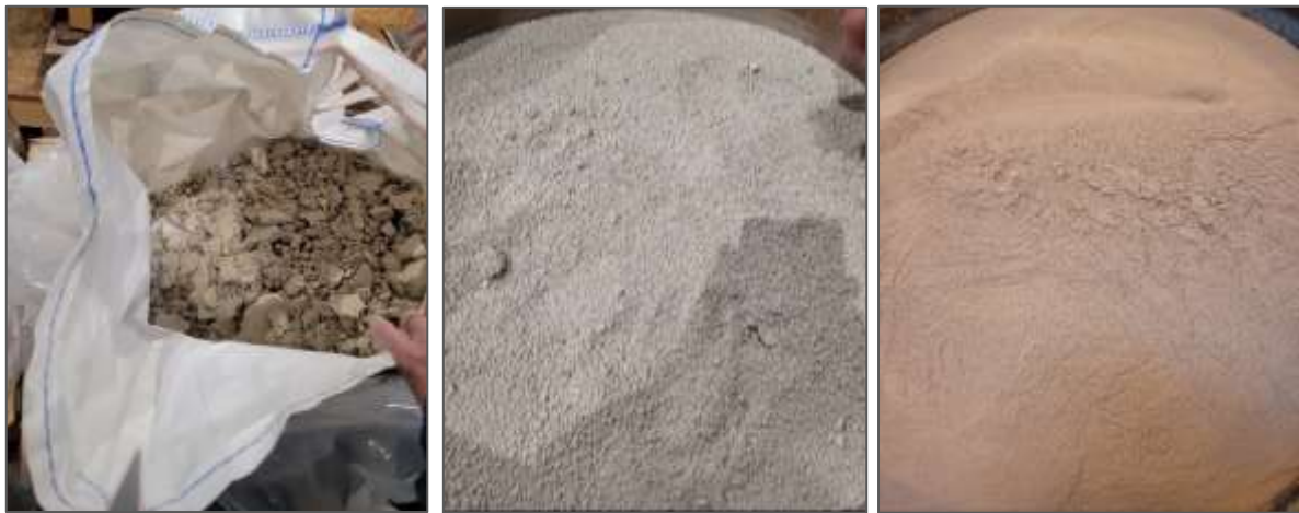
Figure 3.1 Test reclaimed clay: prior and post calcination and ground
