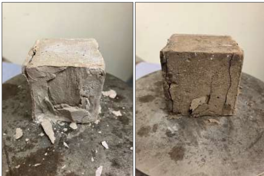
Figure 4.10 CC2F (left) and CC9F (right) normal failure at 34 days.
