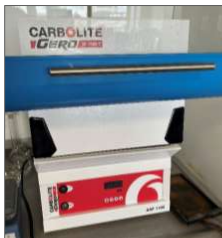
Figure 3.2 Ashing furnace used to calcine FPC clay
