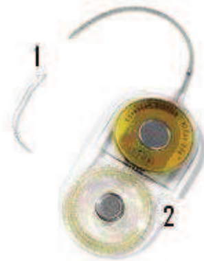
Figure 8: Partie interne d'un implant cochléaire – Marque Advanced Bionic® ( http://www.bionicear-europe.com/UserFiles/Image/Products/90K.jpg )
