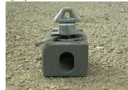
Fig.52: coin ISO et twist-lock.
