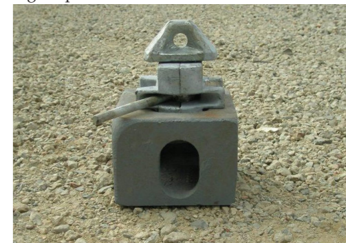
Fig.52: coin ISO et twist-lock.
