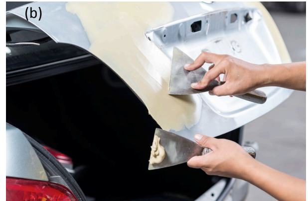
Figure 2 : (a) Mélange du mastic. (b) Application du mastic.
