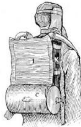
Fig. 33 I. Breathing bag. C. Oxygen cylinder. K. CO 2 absorbent chamber.
